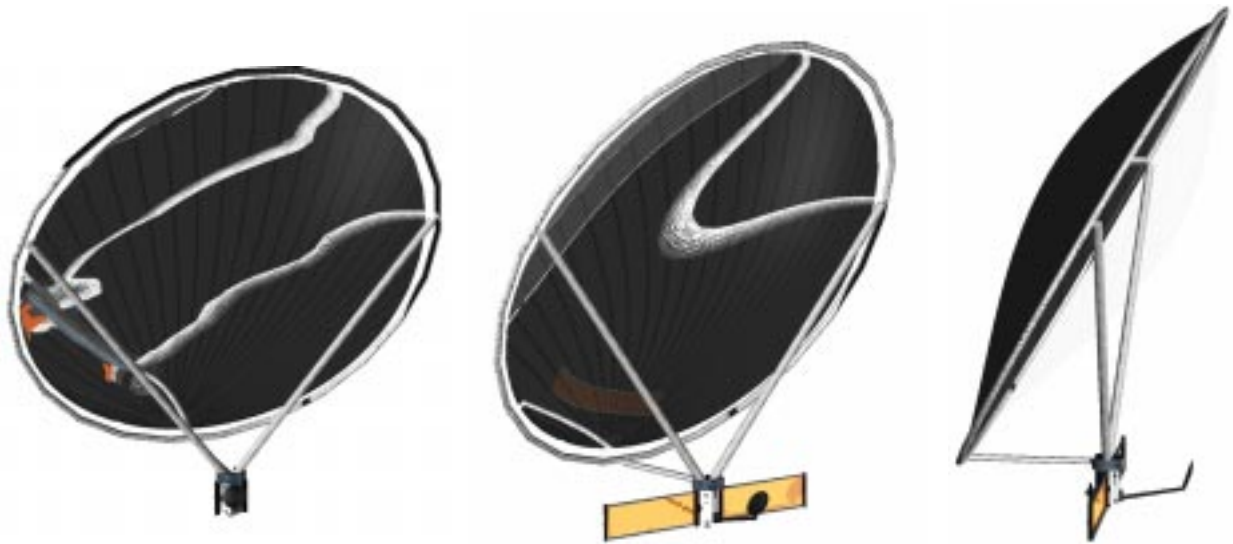
Figure 4.11. Inflation Antenna Deployment Sequence (by TDM Inc.) (continued)
