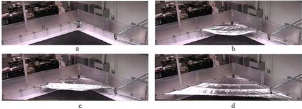
Figure 18. 10 m Sail Quadrant Deployment
