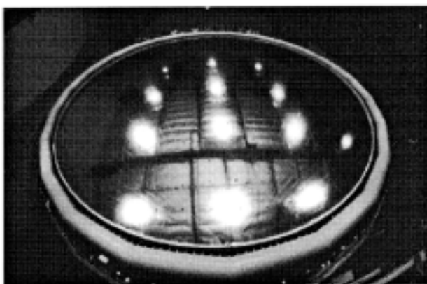
Figure 3. - Ground Test Configuration of the 14-meter diameter inflated reflector for surface accuracy measurement
